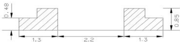
Recommended soldering pad design
