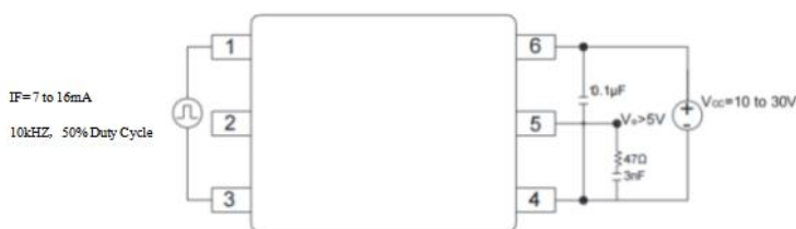
Figure 19: t_{PLH} , t_{PHL} , t_r , and t_f Test Circuit Waveforms
